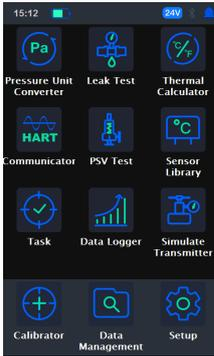
The onboard applications provide a useful selection of features including HART communicator, high static differential pressure mode, pressure leak test, safety valve test, analog transmitter calibration, unit converter, thermal calculator, and snapshots to name a few.
