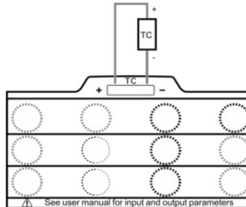
Figure 8 Thermocouple measurement
